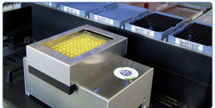
Figure 2: Setup for multiprobe volume verification: integrated balance on the deck of the STAR system
